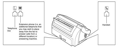
Be sure to connect any external device before using the fax.
